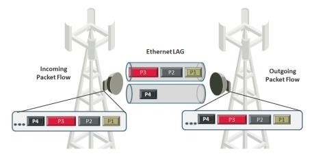
Figure 1: LAG traffic distribution across multiple wireless links
