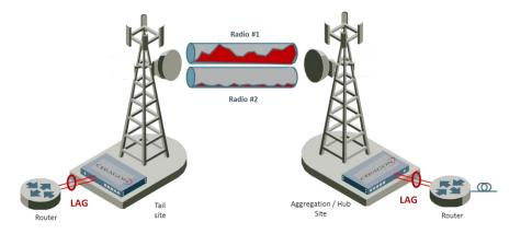
Figure 2: LAG-based wireless link aggregation with common MAC addresses
