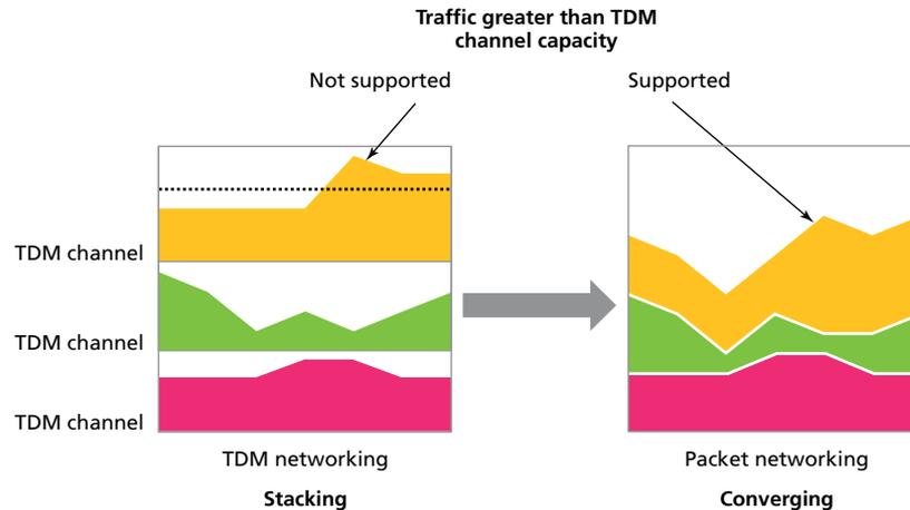
New Packet Optical Transport Systems and microwave packet radios offer resiliency, increased bandwidth capacity, effectiveness and flexibility to allow true network convergence. WDM is added in areas where fiber capacity is exhausted to cost-effectively increase bandwidth capacity. The addition of Zero Touch Photonics capabilities further simplifies WAN operations.
