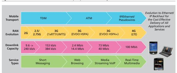
Figure 1. Evolution of the Radio Access Network (RAN) and Mobile Transport Network
