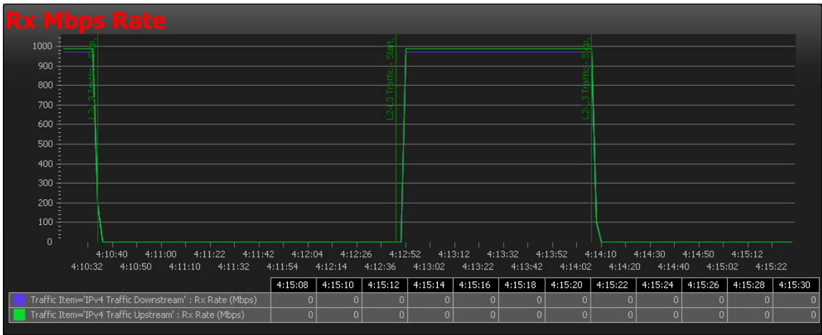
Figure 11. Verify upstream and downstream traffic Rx rate as traffic is started and stopped
